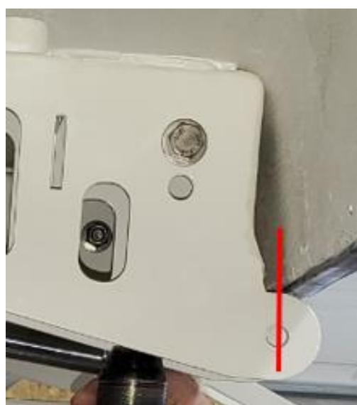
Trace the outline of the chassis as well as the position of the 6 fixing holes under the platform using a marker. The fixing plates (30, 31), which will be positioned on the top of the platform must be well pressed against the surface.
