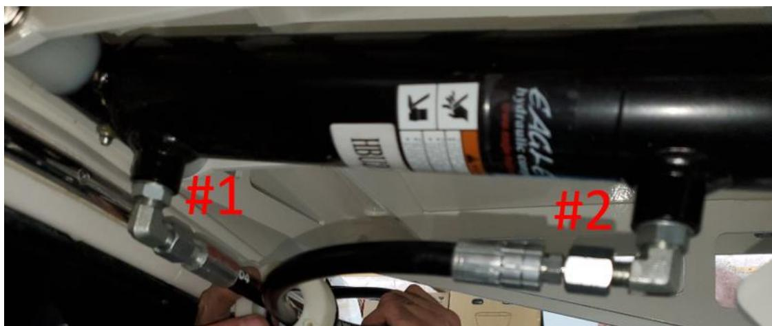
Connector # 1 can be rotated 90 ° by unscrewing the lock nut. **Always unscrew the connector to place it at the desired angle.**
