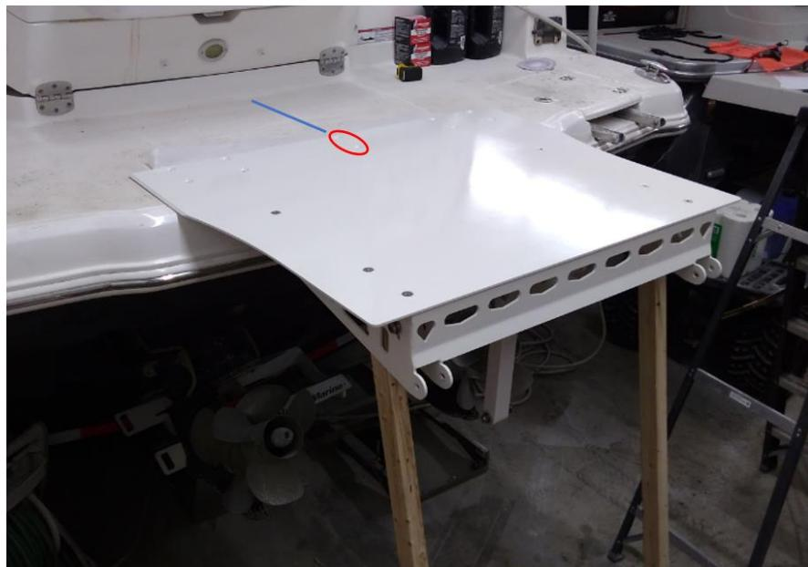
In order to hold the extension plate (20) in place, it is recommended to install temporary posts under the frame (10). If needed, the angle of the extension plate can be adjusted by moving the posts.
