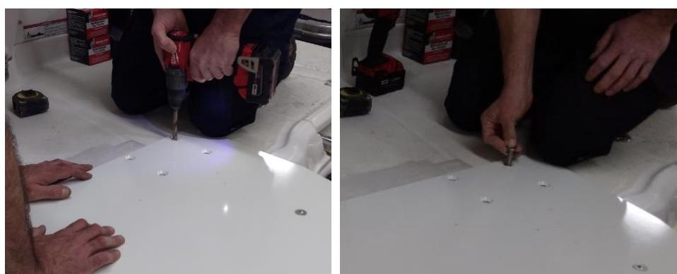
The extension plate (20) now being held in its final position, proceed with the drilling of the other holes. **Make sure to drill only the holes that are required by the chosen mounting option.**
